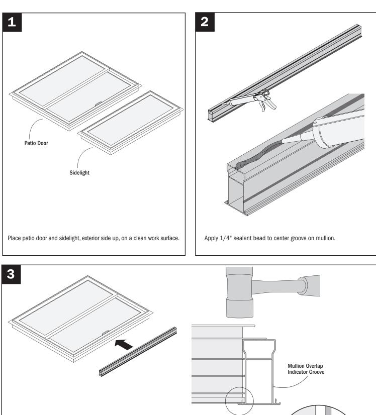
Lift the side of the patio door that will be joined slightly and place the mullion leg against the accessory kerf on the interior facing side of the side jamb. Align the mullion with the edge of the head jamb and sill and set full length using a rubber mallet.
