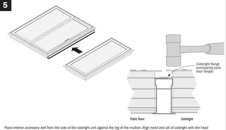
Place interior accessory kerf from the side of the sidelight unit against the leg of the mullion. Align head and sill of sidelight with the head and sill of patio door and set the sidelight on the mullion full length using a rubber mallet. The nailing flange of the sidelight must overlap the nailing flange of the patio door to the exterior.
