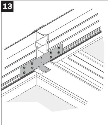
Bend gusset plate tabs inward. Tabs will be bent out and fastened to rough opening during installation.
