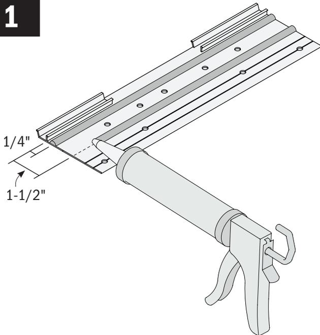
Apply two 1/4" beads of sealant to the sill attachment plate(s), full width, as shown.
