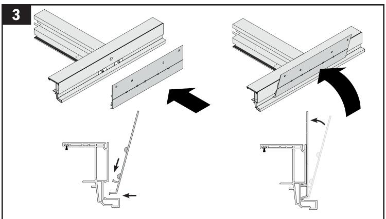
Apply sill attachment plate(s) by inserting the front leg of the sill attachment plate(s) into the channel of the frame's masonry flange at a slight angle. Rotate the sill attachment plate(s) until the back leg snaps into the frame.
