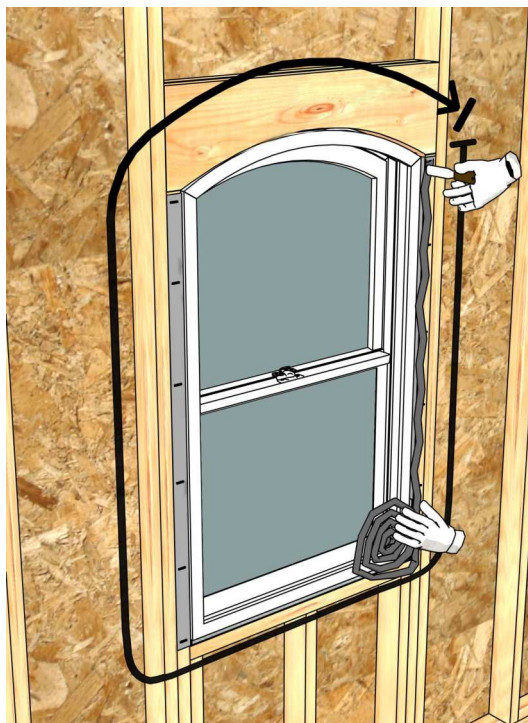
Backer Rod and Sealant Option
