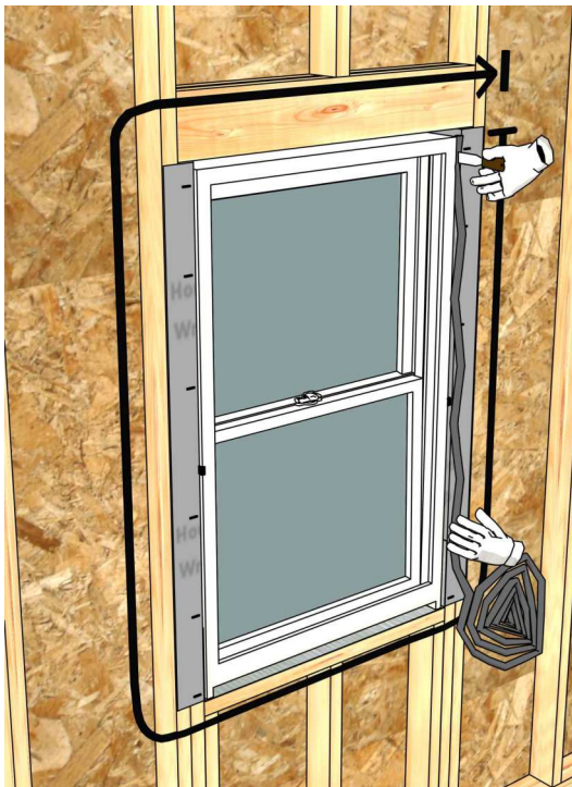
Backer Rod and Sealant Option
