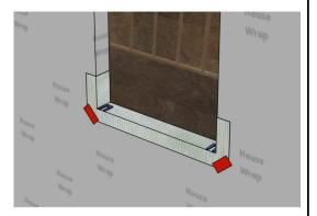
Place shims on the bottom of the opening under the side jamb locations inset 1/4" from each side.
