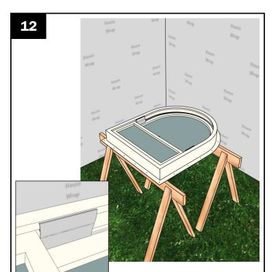
Remove packaging materials except for sash clips. Leave sash clips in place until instructed to remove. Verify that sash are closed and locked.
