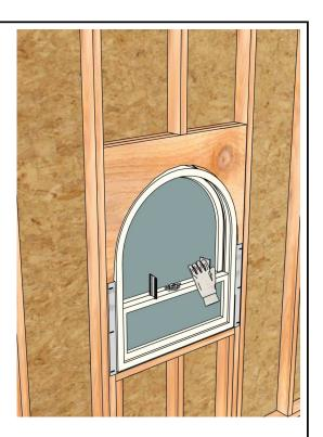
Remove the sash clips. Check for proper window operation.
