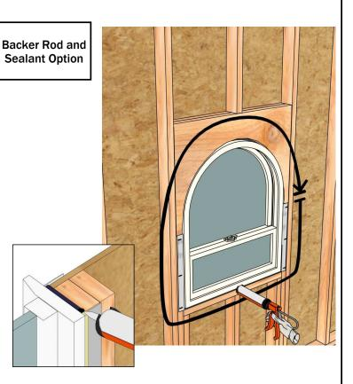
Apply sealant continuously to full perimeter of opening, filling interior 1/3 of cavity as shown using low expanding foam or backer rod and sealant.
