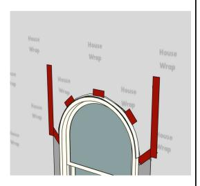
Unfold the house wrap top flap and tape the seams using house wrap tape as shown.  $\,$
