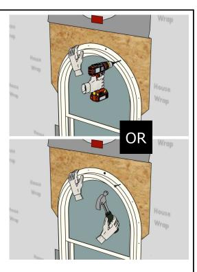
Fasten through the installation flanges. See fastener chart for spacing and approved fasteners.
