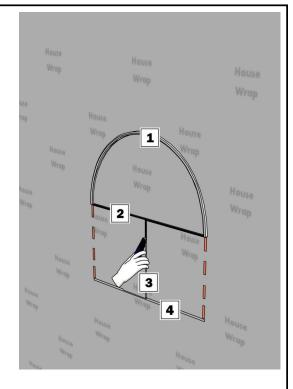
Apply the house wrap according to the manufacturer's instructions and cut opening as shown.
