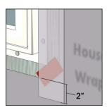
Apply flashing at the sides of the window, overlapping sill flashing as shown. Smooth using a J-roller.
