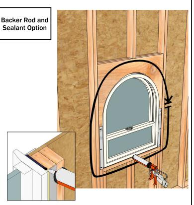
Apply sealant continuously to full perimeter of opening, filling interior 1/3 of cavity as shown using low expanding foam or backer rod and sealant.
