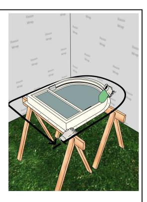
Place window on a clean work surface. Clean the installation flange on both sides using soap and water, or a non-abrasive solvent free cleaner.
