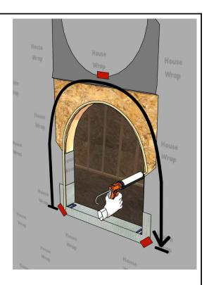
Apply a 1/4" sealant bead at the top and the sides of the opening, no more than 1/2" from the edge as shown.
