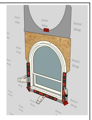
Check that the frame is plumb and level. Adjust shims as needed.
