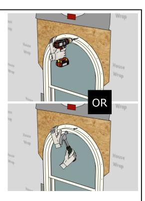
Temporarily fasten with a single fastener at top as shown.
