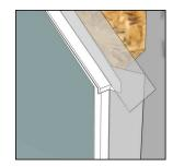
Apply flashing at the head (over the drip cap leg if present), overlapping the side flashing as shown. Smooth using a J-roller.
