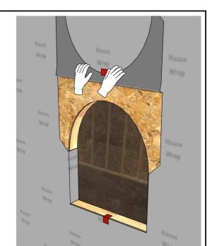
Fold the house wrap flap up and temporarily tape it in place.
