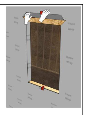
Fold the house wrap flap up and temporarily tape it in place.
