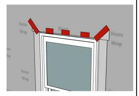
Unfold the house wrap top flap and tape the seams using house wrap tape as shown.  $\,$
