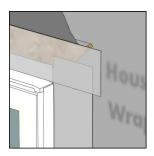
Apply flashing at the head (over the drip cap leg if present), overlapping the side flashing as shown. Smooth using a J-roller.
