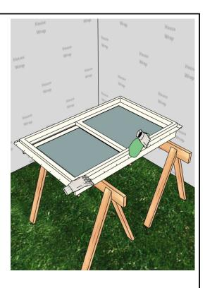
Place window on a clean work surface. Clean the installation flange on both sides using soap and water, or a non-abrasive solvent free cleaner.
