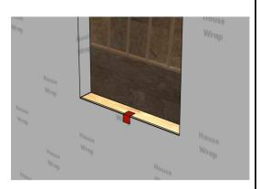
Tape the house wrap at the bottom of the opening as shown.
