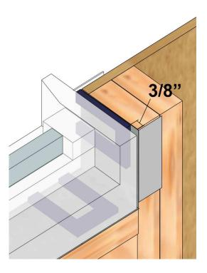
Prepare shims to allow for a 3/8" space for interior sealing as shown.
