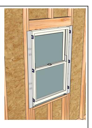
Shim at the sides of the window as space allows using precut shims. Do not over shim.
