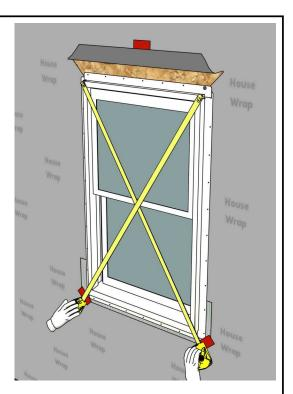
Check that the frame is square. Adjust shims as needed until diagonal measurements are within  $1/8^{\circ}$ .
