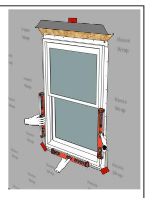
Check that the frame is plumb and level. Adjust shims as needed.
