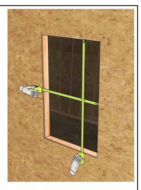
Check that the opening is sized correctly. Allow additional space for flashing thickness, installation clips, joining components, and their fasteners.
