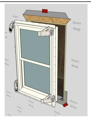
Center the window in the opening, setting the window on the shims. Make sure shims are positioned under the side jambs and integral or joined combination locations as shown.
