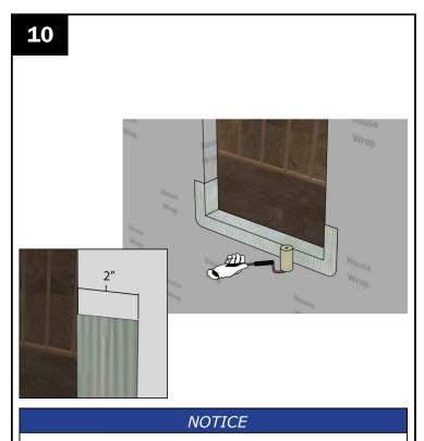
Make sure there are no wrinkles or voids in flashing during application and overlapping. Failure to do so could result in product or property damage.
