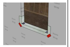
Place shims on the bottom of the opening under the side jamb locations inset  $1/4^{\circ}$  from each side.
