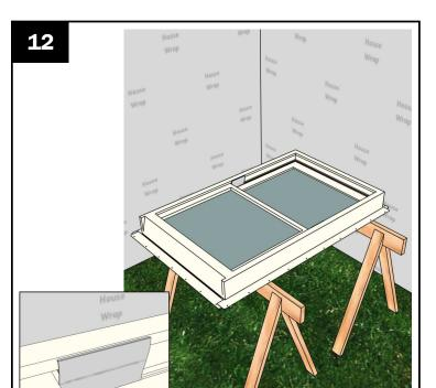
Remove packaging materials except for sash clips. Leave sash clips in place until instructed to remove. Verify that sash are closed and locked.
