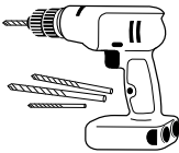
Power driver and 7/32" Drill Bit for Face Mount WOCD or 7/64" Drill Bit for Side Mount WOCD
